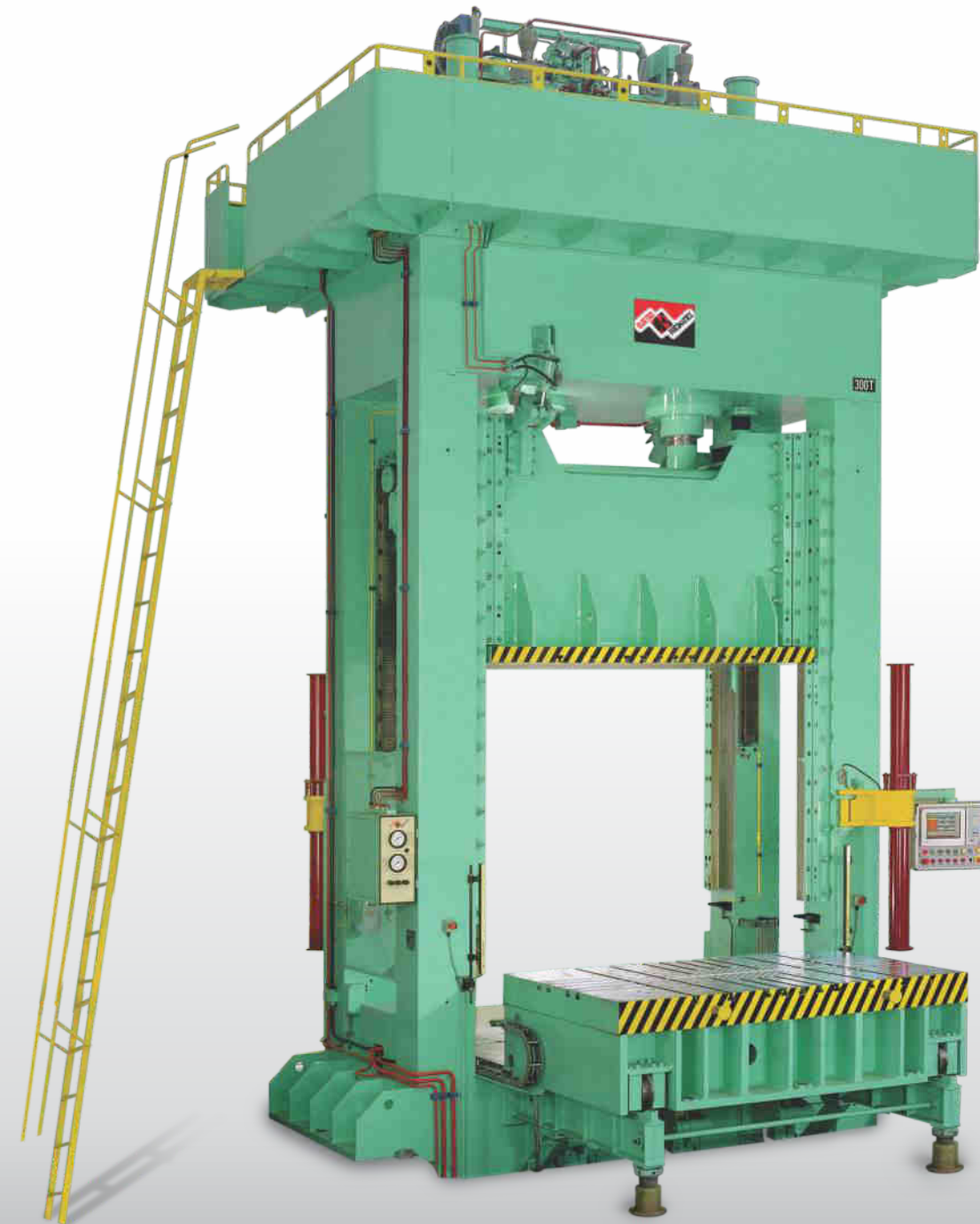
300 T hydraulic die spotting and tryout press with moving bolster, slide equaliser and micro-inching arrangement
