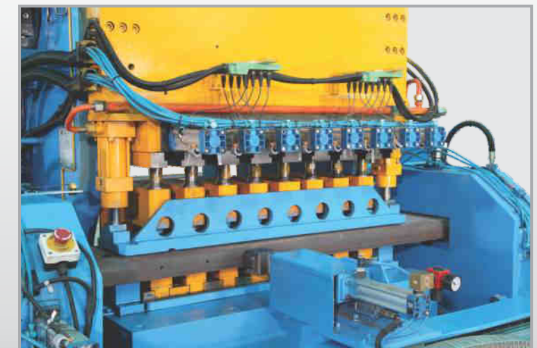
CNC chassis web and flange punching machine with automatic in-feed and out-feed conveyors
