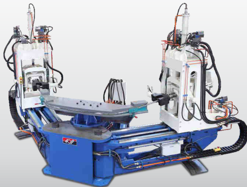
CNC 8-axes hydraulic stretch bender for multi-plane bending of rolled sections
